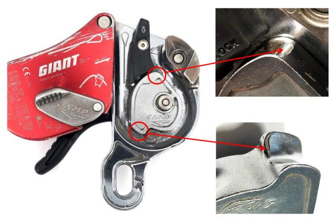
• When, after intensive prolonged use, coating disappears on one or both above shown points, the service life is finished and the descender should be retired.
